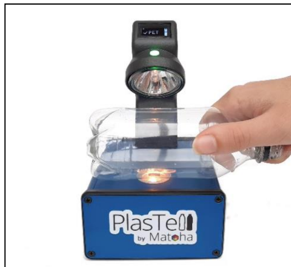
Figure 1: PlasTell, portable plastics analysis scanner
