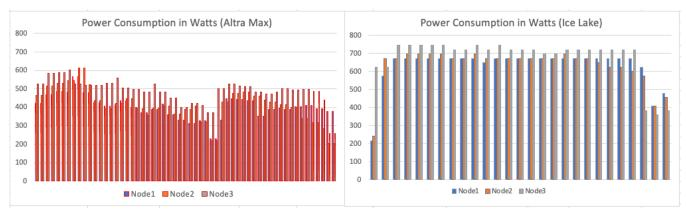
The preceding graphs illustrate the power consumption of the clusters. It is evident that the HPE RL300 servers, equipped with Ampere Altra Max processors, consumed significantly less power compared to the Dell PowerEdge servers featuring Intel Ice Lake processors.
